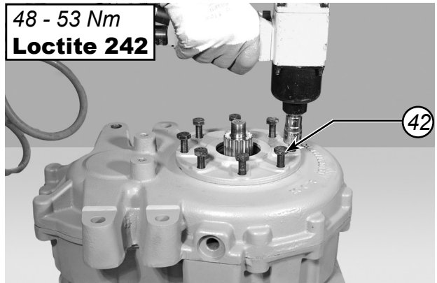
Assembly the screws (42) spreading LOCTITE 242 Tighten screws (42) using a torque wrench setting of 48 - 53 Nm.
